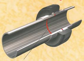
The Clean Joint piping is enclosed in an L-shaped rubber seal. In a sanitary fitting, the pipe abuts a rubber seal. Each provides a smooth internal profile which is free of internal dead spaces. When dead spaces are eliminated the system may be more effectively sanitized which makes it easier to control the growth of bacteria and biofilm.
