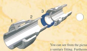
As the nut (1) is tightened, the ferrule (2) grips the pipe and draws it forward against the rubber seal (3). The result is a secure seal without any dead spaces to harbor bacteria and biofilm.
