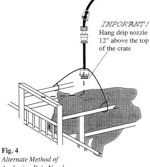
Alternate Method of Anchoring Drip Nozzles
