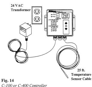
You are now ready to install the Controller and connect it to the system. Whether you are using the C-100 or the C-400 mode Controller, the installation is the same. It should be located where it is readily visible to easily monitor the room temperature readout and easily accessible for programming.
