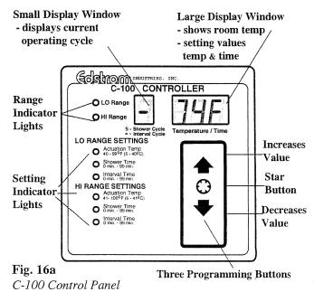
The control panel of the C-100 Controller is shown in Fig. 16a. Digital displays and indicator lights indicate the operating status of the unit. Three programming buttons are used for viewing all the programmed setting values and making any desired changes to the settings.
