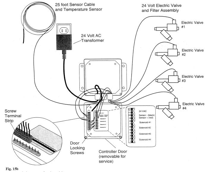
C-400 with door open showing wiring
