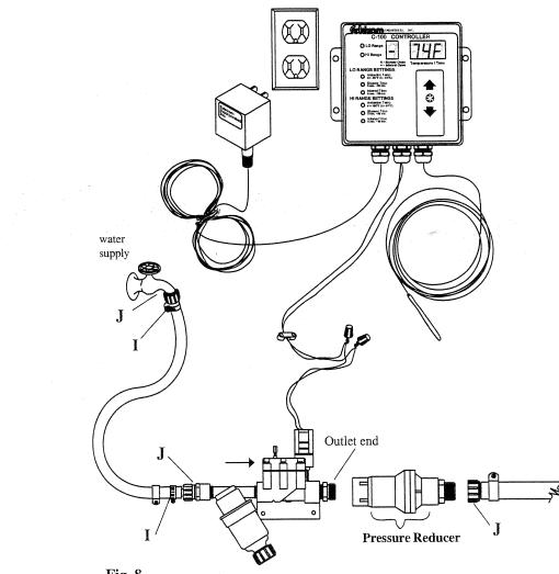
Fig. 8 C-100 Controller, 7400-8951-015 Electric Valve/Filter, 7400-8945-550 Pressure Reducer, 2100-5234-015
