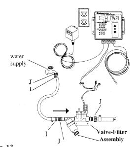
Fig. 13 C-100 or C-400 Controller Electric Valve/Filter, 7400-8945-140
