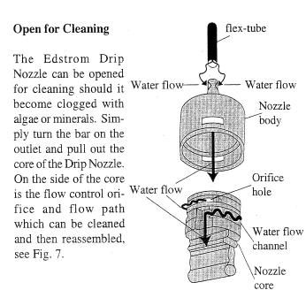
**Fig. 7** Drip Nozzle - exploded view
